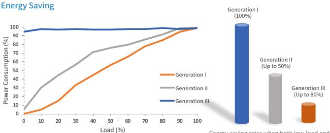
Energy-saving rates when both low-load and no-load conditions are considered
