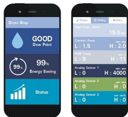
Monitoring unit by mobile phone
