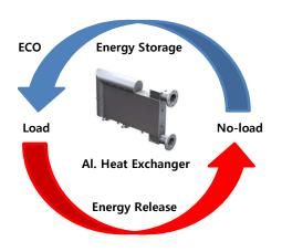
GSA's 2<sup>nd</sup> generation Cycling refrigerated air dryer includes the basic refrigerant circuit of 1<sup>st</sup> generation refrigeration dryer. It saves energy by stopping the refrigeration dryer by controlling the cooling energy and temperature stored in the heat exchanger when there is no load or low load.
